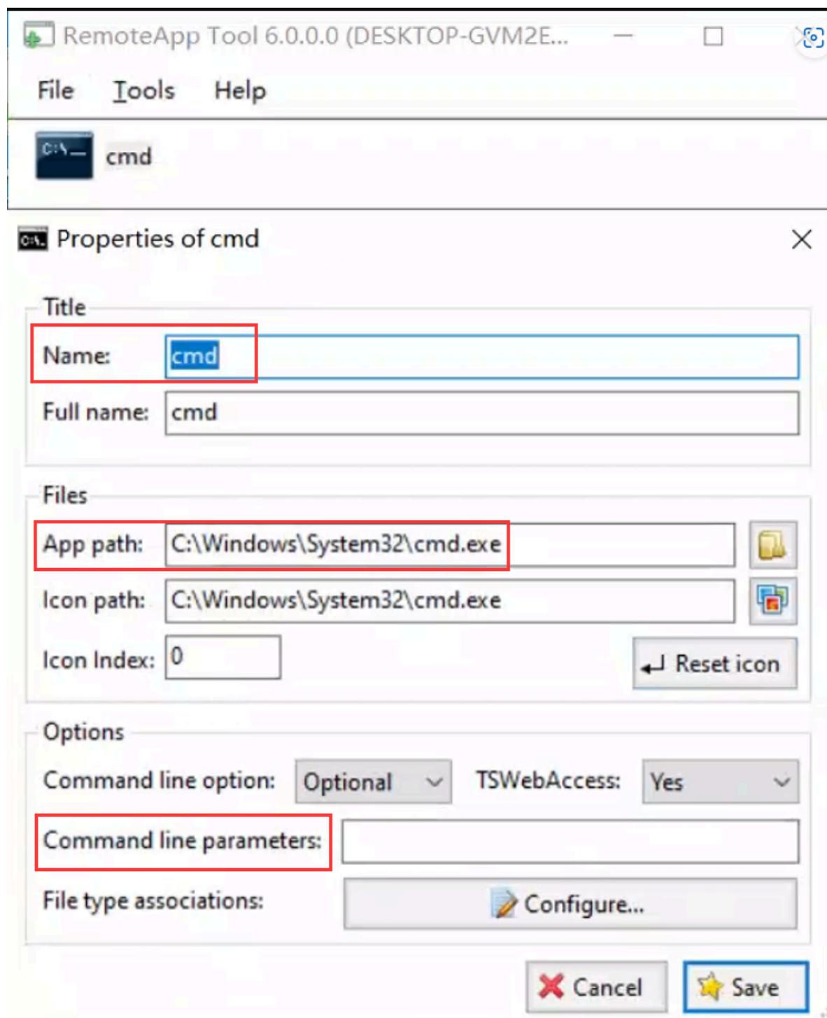
2. Configure the remote app information in the asset edit page according to the server-end configuration. 'remoteAppName', 'remoteAppDir', and 'remoteAppArgs' are required.
